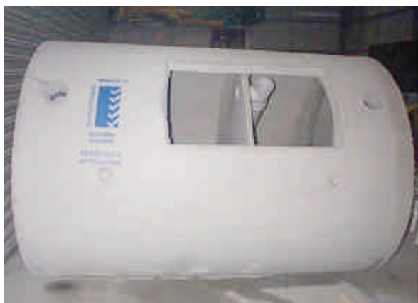
Photo of one type of AWTS concrete tank.
