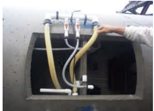
An AWTS showing some of the internal components on display outside the tank before installation.
