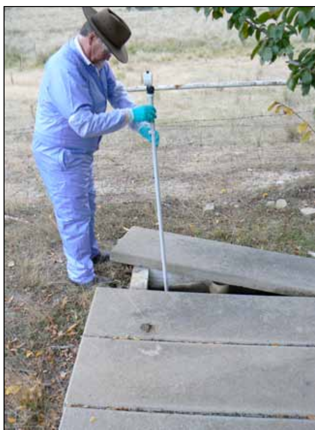
Figure 4.6 Testing sludge depth using a ‘Sonic Sludge Stick’
